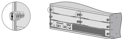
2. Pull out the line card levers and carefully slide the line card halfway out of the slot. If you are removing a blank line card, pull the blank line card completely out of the chassis slot.
